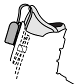
Adequate Power Cord Exposed
